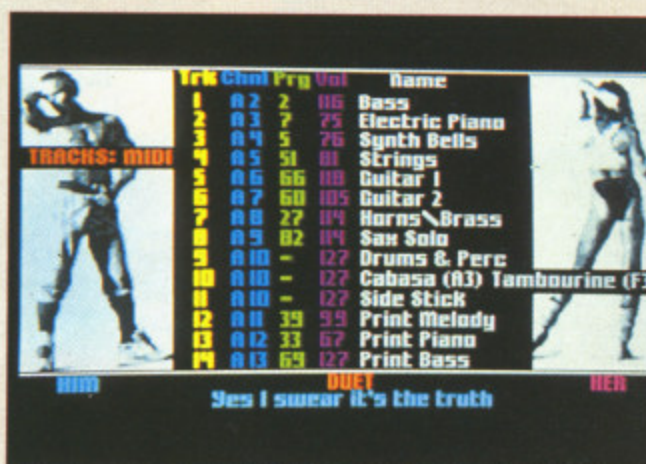
CD+G enables you to display simple graphics and text while your commercial CD+G audio disk is playing. In this case it's being used with the CD+G+MIDI function, showing you which MIDI channels are being used by the current disk and - at the bottom - which vocals are being sung. Result - you can not only sing along Karaoke style but can also change the orchestration by feeding the MIDI track into your synth and getting CD audio, synth, and your own voice all working together!
